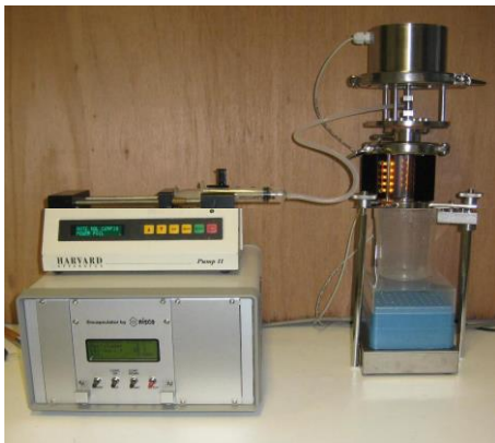
Figure 1. The Nisco Encapsulator used to fabricate the microspheres being evaluated in the project. The encapsulator consists of a vibration unit and control cabinet. Polymer solution is fed into the vibration unit via a syringe pump before being dropped into a container holding liquid nitrogen. A stroboscopic unit facilitates visualization of the droplets.
